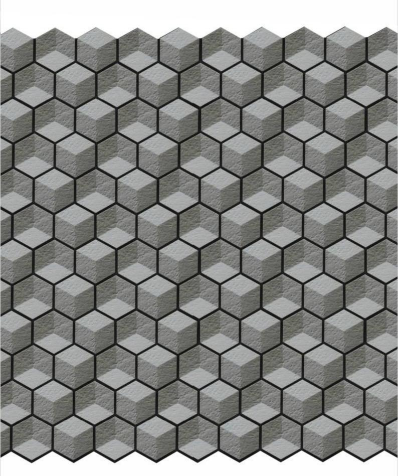
StoneWiz wall panels & 3-D perspective tiles are manufactured using state of the art Ultra High Performance Fiber Reinforced Concrete (UHPFRC). UHPFRC has characteristics of high compressive strength (90-120 MPA), high flexural strength (10-15 MPA) & very low porosity which is achieved by our proprietary formulation of precisely measured ratios of finely graded materials.
